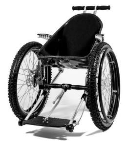
Like most modern vehicles, we've done away with the traditional metal chassis and replaced it with a super lightweight carbon fibre seat. This reduces the weight of the chair, whilst keeping it strong. In a recent customer survey, 87% of people said their Trekinetic wheelchair had given them more independence.
