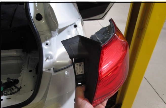
Remove the right hand rear light cluster then mark and drill a 10mm where shown for the
