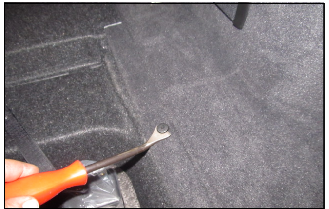
Remove the pins securing the side cover then remove the side cover
