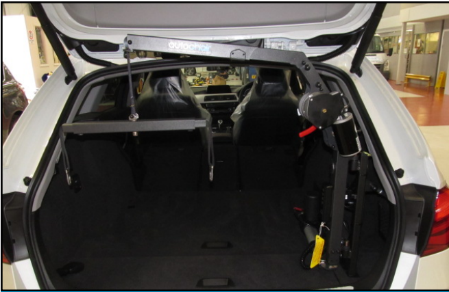
Assemble the Hoist and adjust to suit the application. Power should be taken direct...
