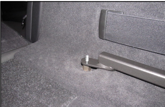
Locate the front mounting of the frame onto the spacer
