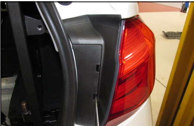
Remove the right hand rear light cluster then mark and drill a 10mm where shown for the
