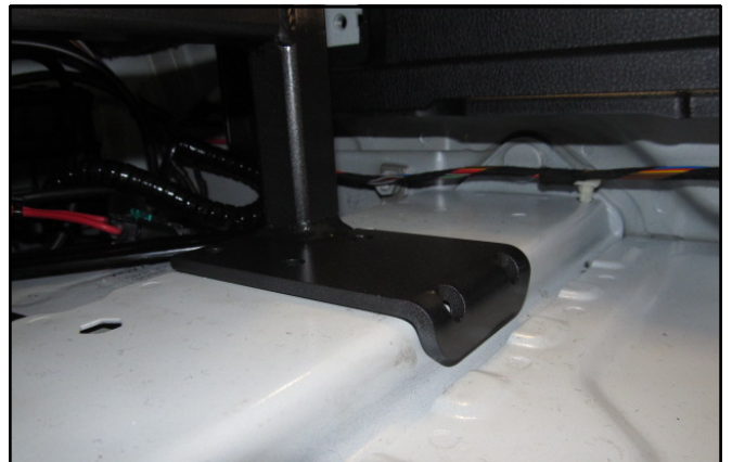
Position the rear mounting as shown and drill the hole shown to 9mm
