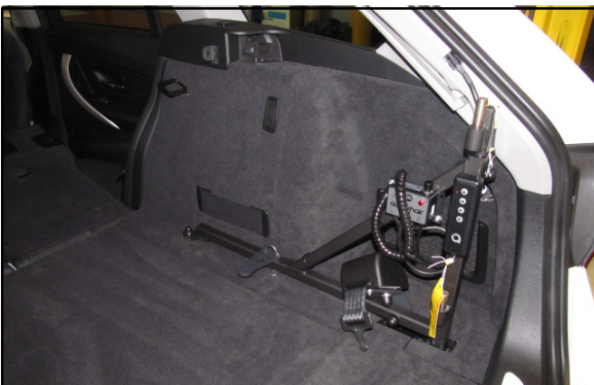
Place the frame back in position and fully secure all 3 mountings. Trim and refit the floor covers
