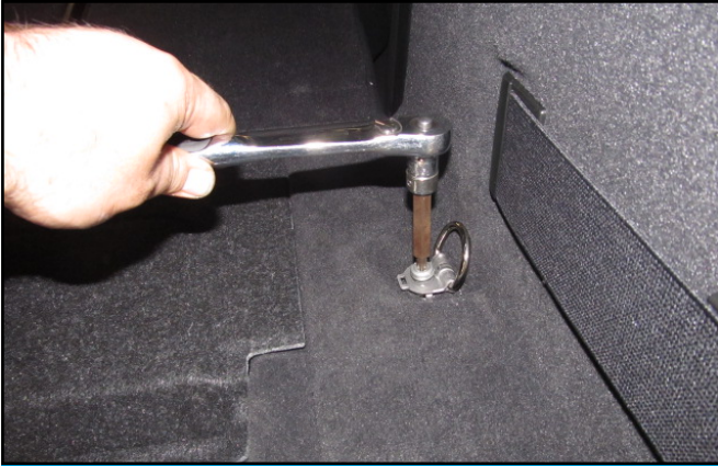
Unscrew and remove the front right hand luggage tie down lug
