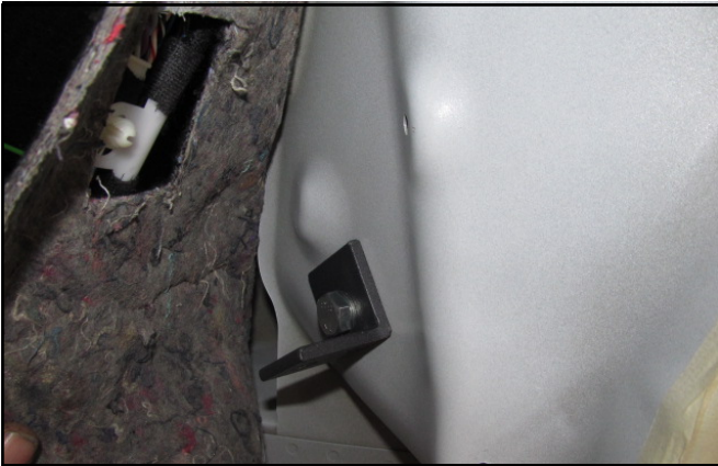
Fit the bracket shown on the inside of the vehicle tightening it from the outside
