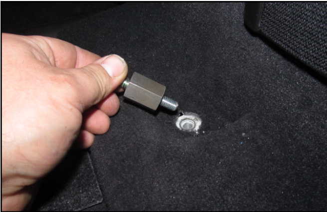
Temporarily remove the spacer for the front mounting to improve access behind side panel
