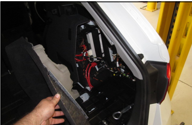
Unscrew then remove the plastic insert
