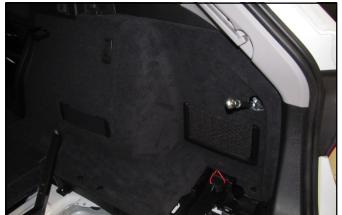
Refit the light cluster then refit the side cover around the bracket
