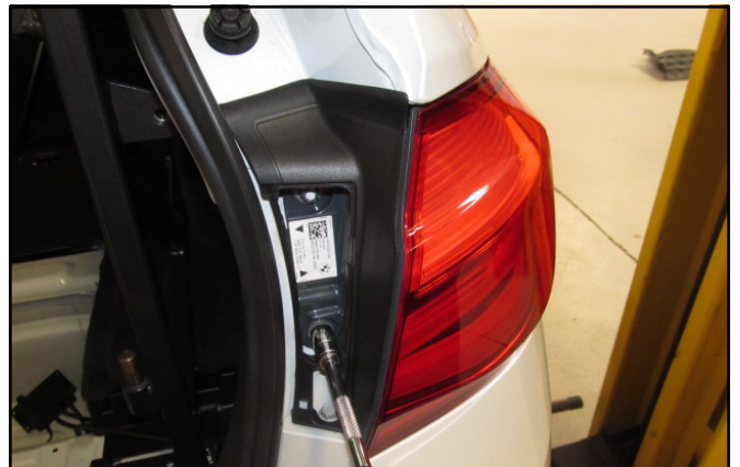
mounting of the spreader plate
