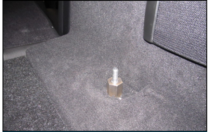
Replace the lug with the hexagon spacer with studding shown
