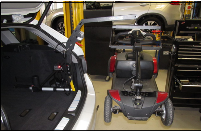
Assemble the Hoist and adjust to suit the application. Power should be taken direct...
