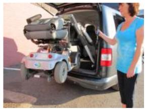
Transferring a scooter, powerchair or wheelchair into a vehicle with Autochair (200kg capacity shown).
