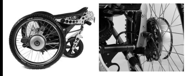
The Trekinetic GTE was designed to fold down and fit into a regular car. The front wheels come off with the simple click of a button and the rear castor folds down behind the seat. It has also been designed to fit into most larger vehicles with the wheels still on.
